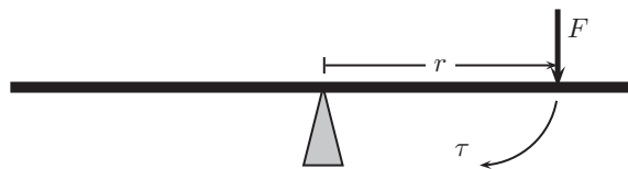
Figure 12.17: The force exerted on one side of a see-saw causes it to swing.
